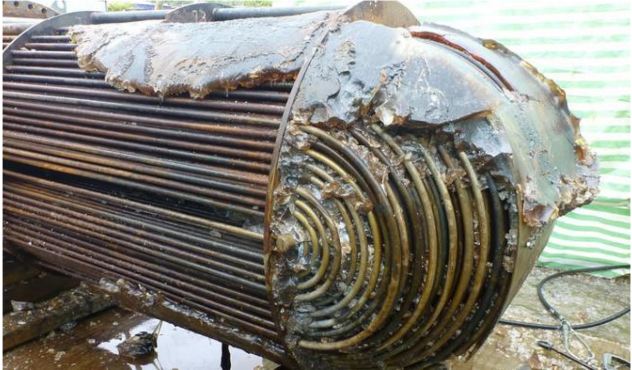
Figure 17: Shell side fouling in a petrochemical heat exchanger
